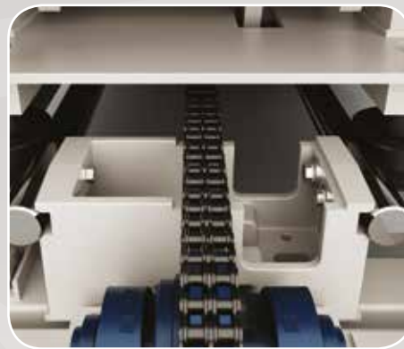
Guide del carro porta lama Slideways of the blade holder carriage Guides du chariot porte-lame Guías del carro porta-hoja
